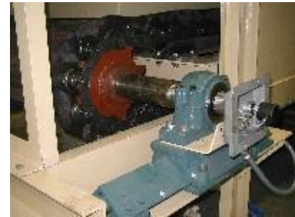
Tail sprocket, take-up, bearing, shaft and speed sensor (cover removed)
